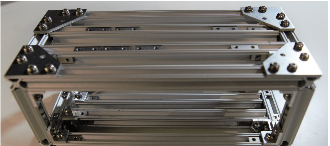
Figure 38. Addition of the top plate, view 2
