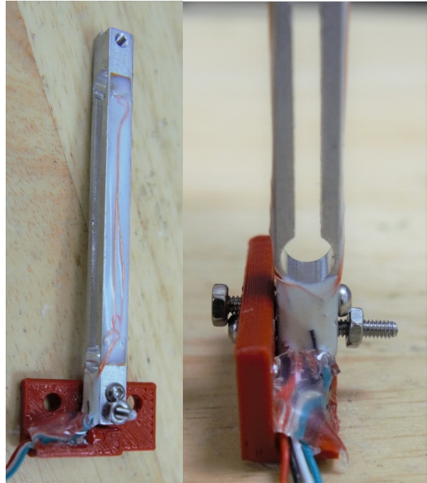
Figure 13. Strain gauge mounted on the strain gauge sidewall
