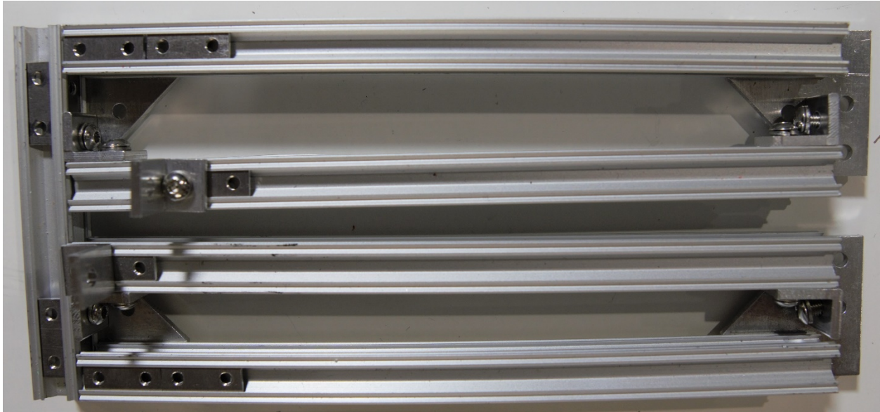
Figure 25. Assembly of outer and mid-runner frames
