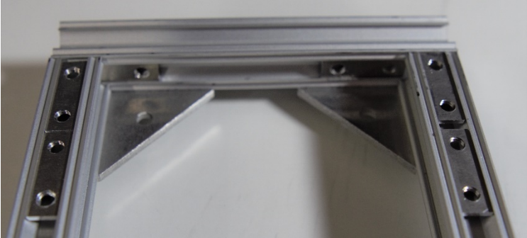
Figure 31. Correct installation of sliders on outer frame
