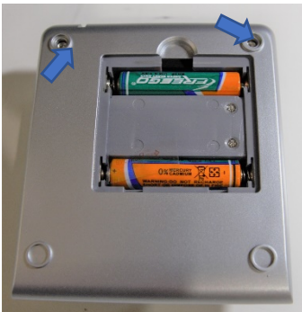
Figure 2. Screws and batteries to be removed
