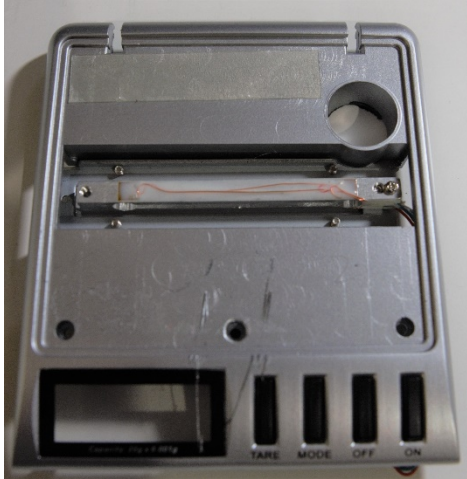
Figure 9. Donor scale with weight plate removed
