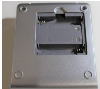
Figure 3. Screws and batteries removed
