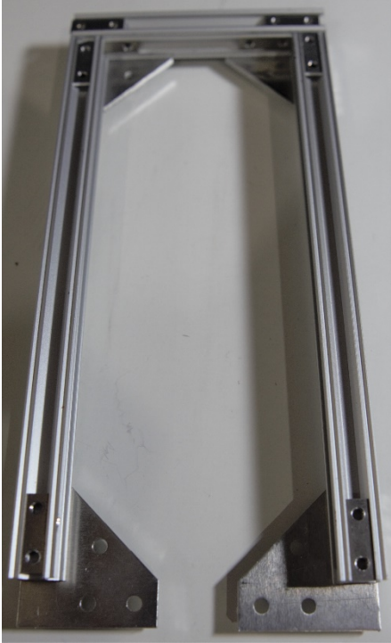
Figure 30. Outer frame, final assembly
