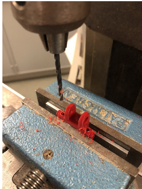
Figure 39. Drilling holes for the 3mm shafts
