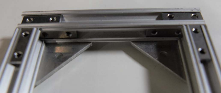
Figure 24. Correct positioning of sliders
