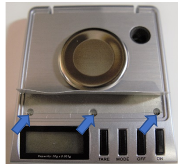
Figure 4. Revealing hidden screws
