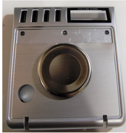
Figure 7. Removal of scored section of top plate
