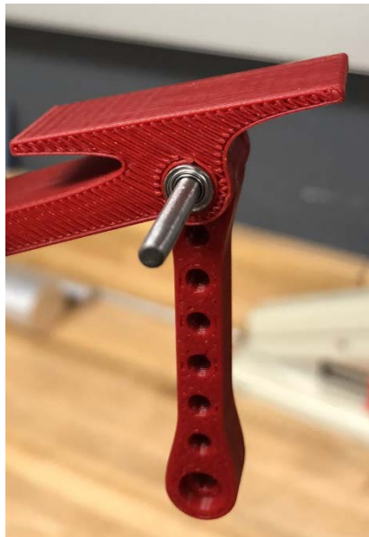
Figure 41. Verifying that the links hang freely
