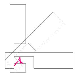
The next step is to constrain the positions of link BC relative to each cabinet door position. To do this, 3 lines are needed. I chose to use the end corners of the cabinet doors as a reference point. Shown below are the 3 lines drawn connecting each link BC to the correct cabinet door.
