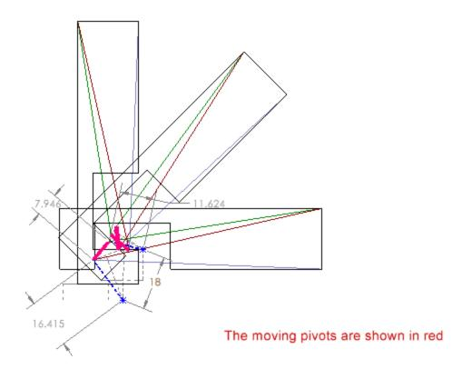
The scale shown here is 1:1, and the complete solid works drawing is attached below. To get the project to fit nicely on the given wood material, I divided the calculated lengths by 4 and changed the units from mm to in. The ground pins are shown by the blue "\*" points.
