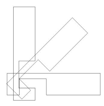
The next step is to arbitrarily draw the link BC, with its correct length at each position. These lines should not have their position relative to the cabinet door dimensioned as that comes later. Shown below is the link BC drawn at each position.
